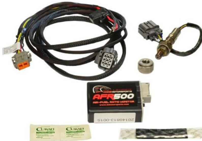
Troubleshooting problems are simple. If your meter reads rich but the engine has signs of being lean the sensor is probably plugged from lack of preheating or is worn out. Readings that bounce around or show false lean are usually caused by air flow reversion because your sensor is too close to the exhaust tip or there is an air leak between the engine and sensor.
