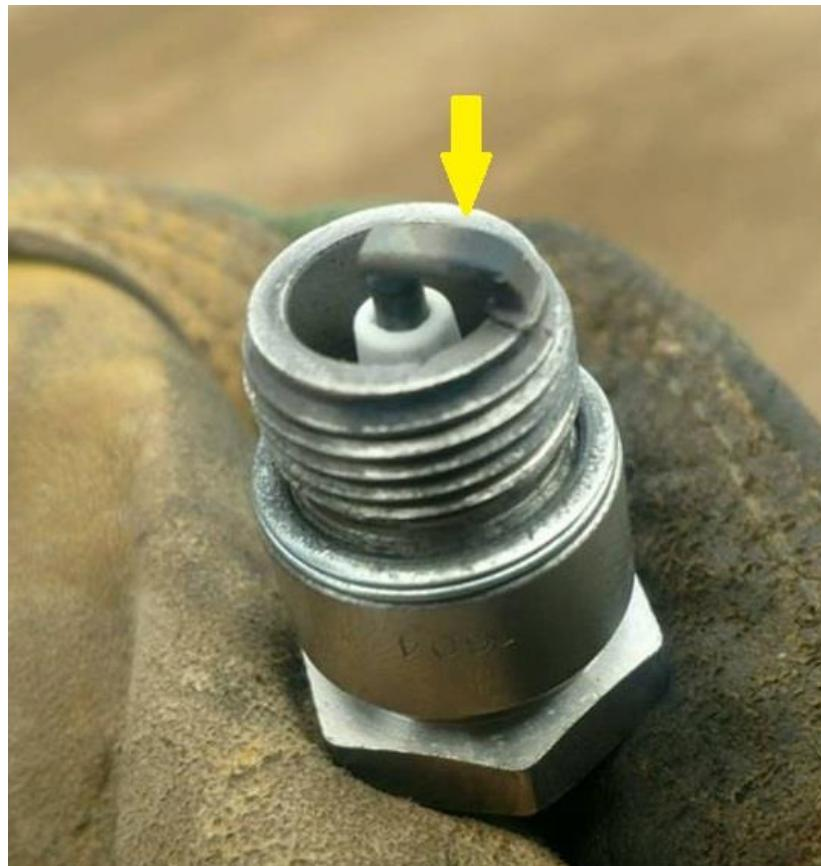
Much like a knife maker who looks for the proper “temper line” to read metal temperature, we can use the same method to read spark plugs. As your plug heats up, a color line begins to form on the ground strap. Even if your spark plug has carbon soot, you can carefully wipe the plug clean and read the color change of the metal.
