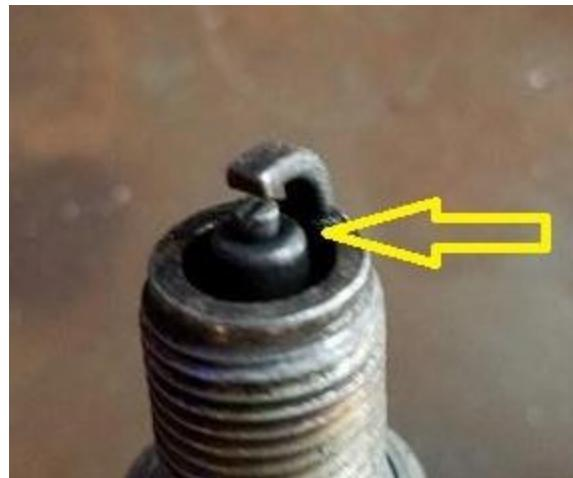
Black specs on the insulator indicates detonation, silver specs indicate piston damage from extreme detonation. Use a magnifying glass and bright light to inspect the insulator down at the base (inside the threaded area). Generally a 2 millimeter wide brown or grey color at the base is acceptable.
