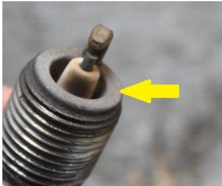
The spark plug shown above has an even light color indicating correct jetting. If you are using certain ignitions such as our C5 multiple spark system the color typically appears lighter than a stock type ignition with a single spark. Using an air-fuel meter to verify jetting is highly recommended and saves time.
