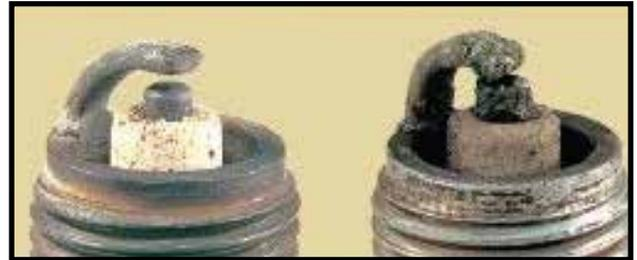
**In my opinion you want the coldest tip possible without fouling. That prevents auto ignition (fuel igniting without spark). Fuel generally needs a spark or concentrated heat source to ignite. The spark plug tip and outer edge of the exhaust valve are two common heat sources that cause auto ignition.**
